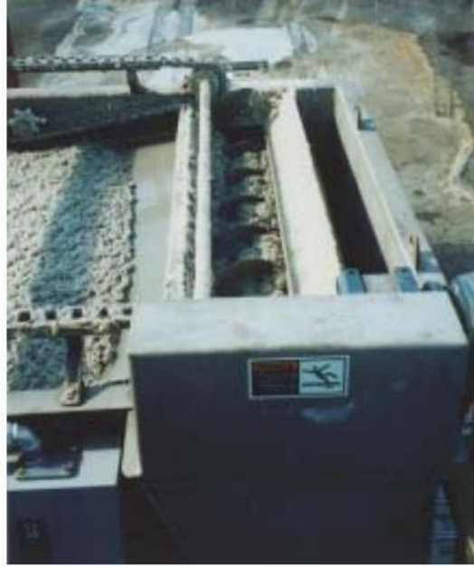
Scrapers move a thick sludge blanket to the auger area.
